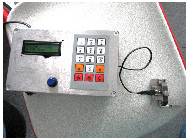
Figure 4. Measurement of pressure applied by the bulldog clamp.
